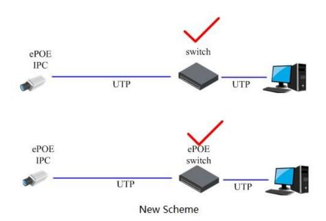
Figure 14 Advantage of ePoE IP System
