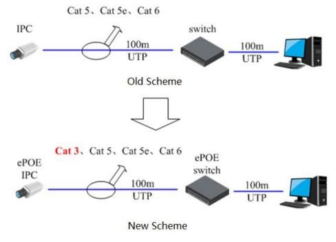
Figure 12 Advantage of ePoE IP System
