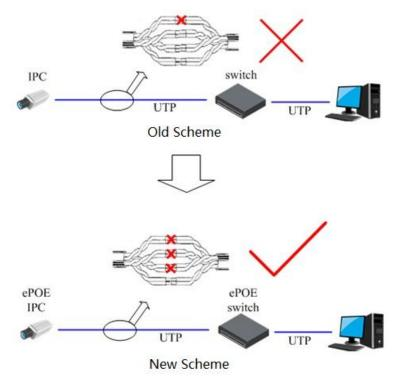
Figure 13 Advantage of ePoE IP System
