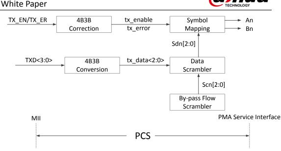
Figure 6 Data Transmission Reference
