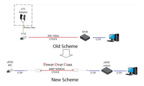
Figure 16 Advantage of ePoE IP System
