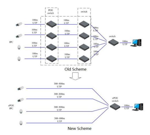
Figure 11 Advantage of ePoE IP System
