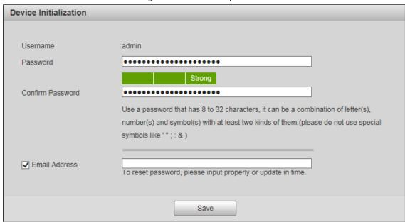
Step 3 (Optional) Set the email address which is used to reset password.
