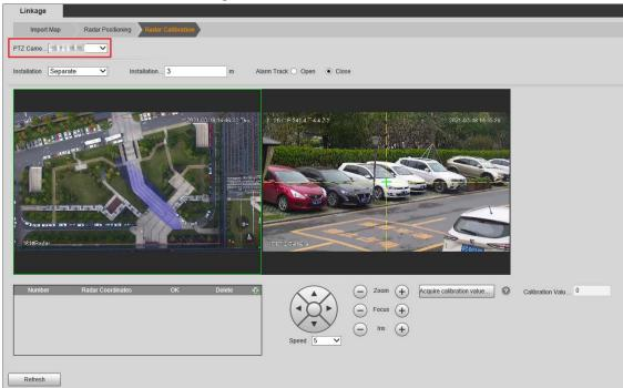
Step 2 Enter the installation height of the camera.
