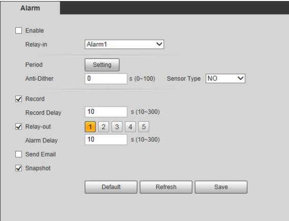
Select **Enable** check box to enable the alarm linkage, and configure parameters as needed. Step 2
