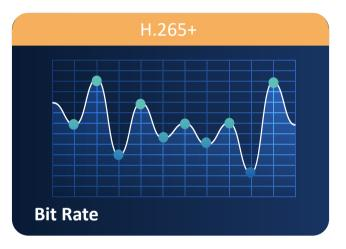
VBR (Variable Bit Rate) has high burstiness, which makes it difficult to calculate the required bandwidth.
