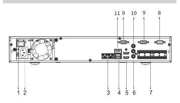
1 Power Switch Power Input 3 Network Ports USB Ports 5 HDMI Ports AUDIO IN, RCA Connector 6 RS-232 Port 7 Alarm In/Out 10 AUDIO OUT, RCA Connector 9 VGA Ports
