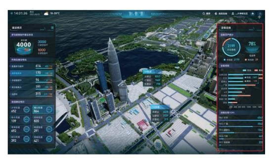
In the equipment operation and maintenance module, we can know the total number of equipment mounted on the smart pole of the current platform and the online rate.
